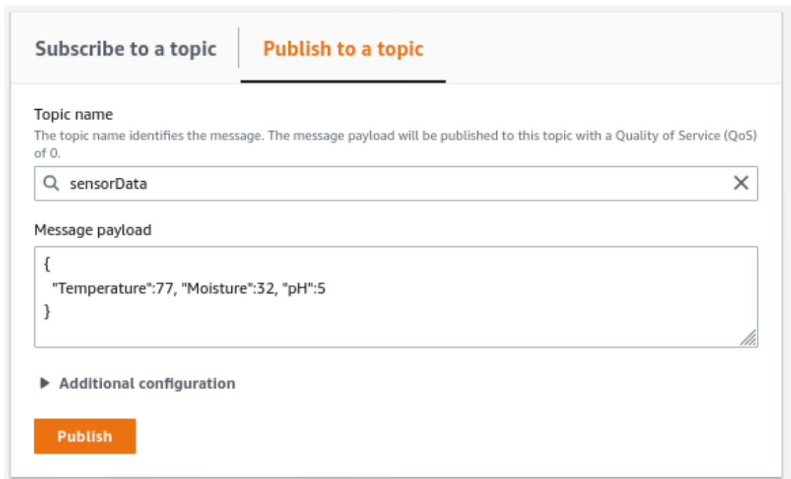
Figure 7: AWS's MQTT Test interface which is publishing the data displayed in Figure 6
